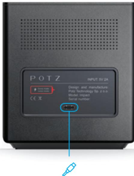
USB-C socket located at the back of the device
